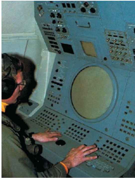
Fig. 16. TACCO & Track Ball (early mouse) Source: US Navy
